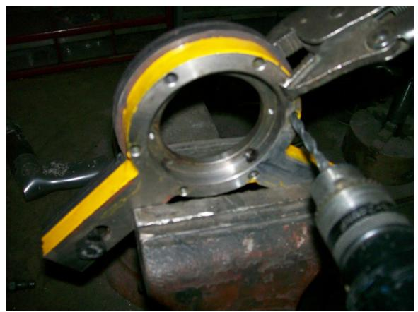
5. Now change to a 4.5 MM drill and drill all the way through both stiffener plates. At the same time drill 2 holes- one on each side of the bolt.
