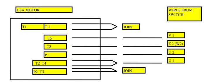
PLEASE NOTE: TO REVERSE MOTOR DIRECTION SWITCH POSITIONS OF T5 AND T8 MOTOR WIRES
