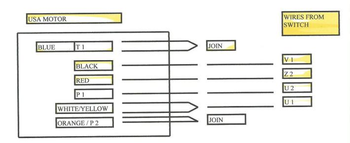
PLEASE NOTE: TO REVERSE MOTOR DIRECTION SWITCH POSITIONS OF RED AND BLACK MOTOR WIRES IF YOUR MILL CABLE IS TOO SHORT, USE THE ENCLOSED PIECE TO EXTEND THE LENGTH.
