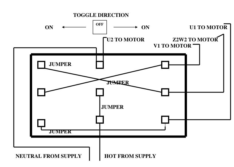
On machines with rotary switches, your toggle switch will fit in the original mounting hole. For machines with push button switches you will need to make a plate to fill the rectangular hole and drill a hole for the toggle switch.
