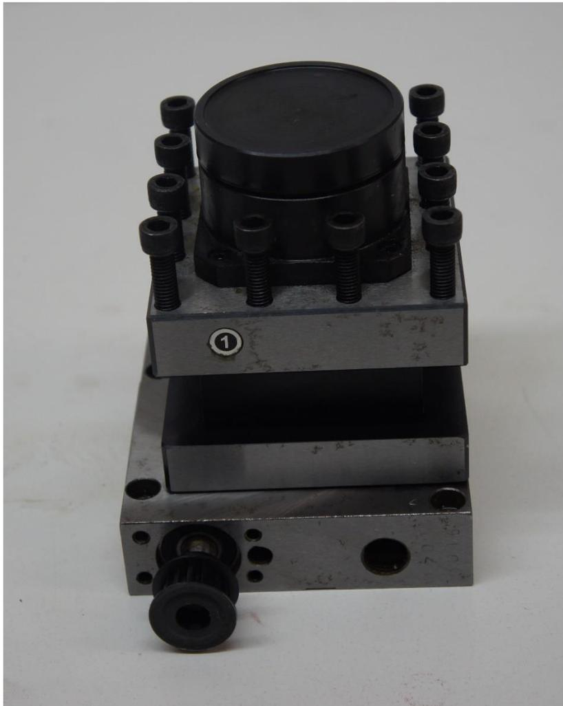
2. Turn the pulley counter clockwise until the turret turns to the 45 degree Position and exposes all four mounting holes. ( this make take quite a few Turns)
