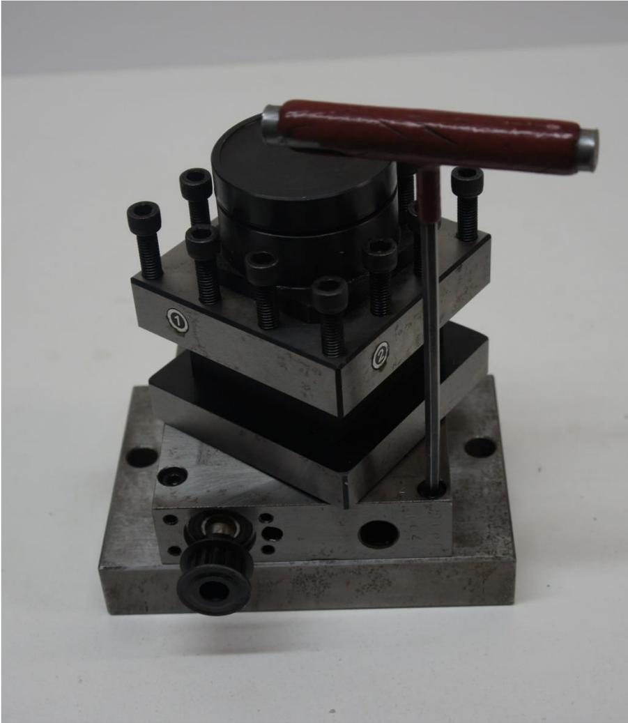
3. Bolt the main center turret to the steel base plate using the 6mm Socket
