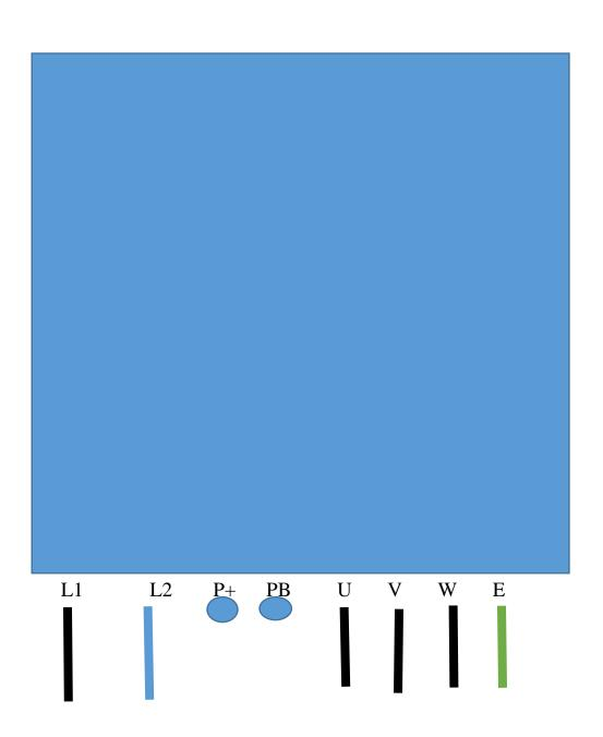
The row of low voltage terminals are only used if you are wiring to a CNC system for computer control of the spindle motor
