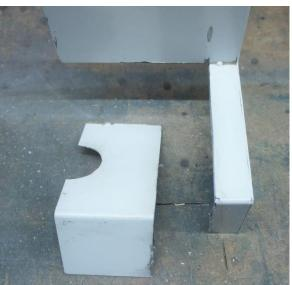
3. Place the mounting bracket on the 3 spacers with the single hole facing the motor. Center the hole in the bracket over the spindle and square the bracket to the mill head casting. Clamp it in place with a "C" clamp and using a transfer punch mark the 3 holes through the spacers. Drill and tap the 3 places to 10 MM X 1.5 threads.
