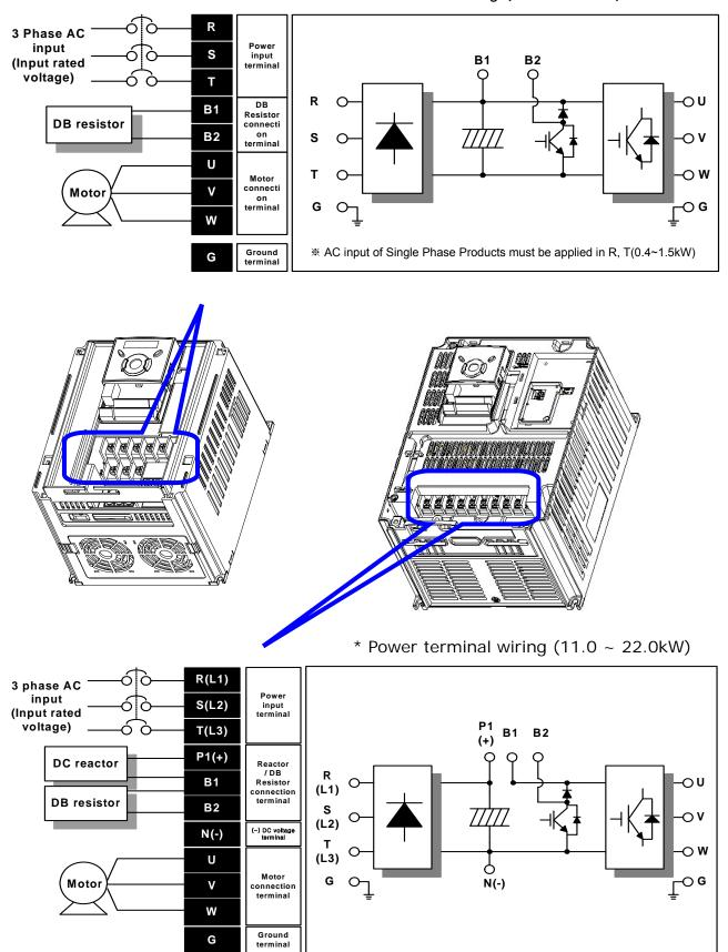
2.4 Specifications for power terminal block wiring
