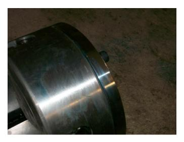
7. Using a transfer punch, punch mark through the other 2 holes in the faceplate into the back of the 4 jaw chuck.
