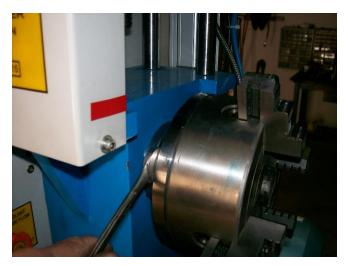
2. You will see that the mill turn has a face plate that is bolted to the spindle with 4 allen bolts-remove the bolts and the face plate.
