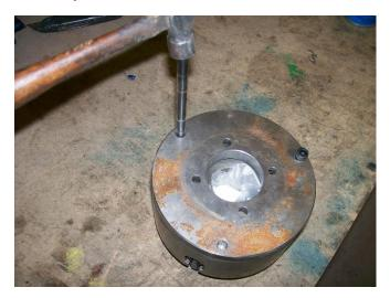
8. Drill these 2 holes with a 7MM or  $9/32^{\prime\prime}$  drill and then tap them to 8MM X 1.25 threads.
