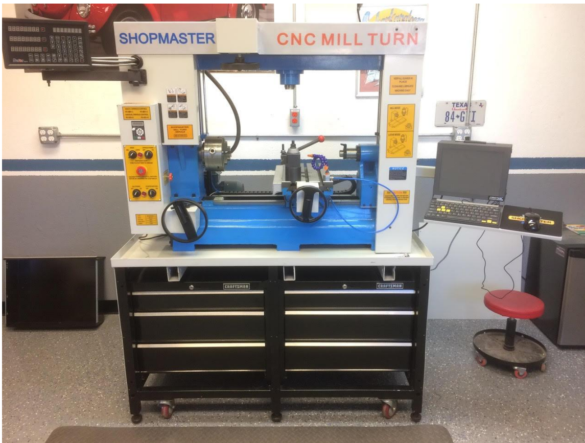
BRIDGEMILL AND TURNADO BENCH ARE THE SAME picture shows doors removed and toolboxes installed
