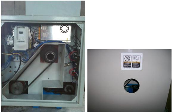
While the end panel is open and power disconnected you should check the drive belt tension, stepper belt tension and adjust any switch knobs that are not properly "clocked".
